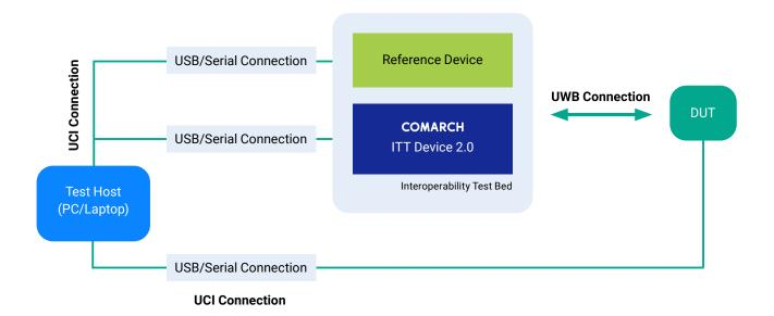
Physical connection for ITT is similar like in the MCTT. This is a plug-and-play solution. The interoperability testbed is made up of the IOP Test Tool (one unit of ITT Device 2.0) and from 1 to 8 reference devices.
