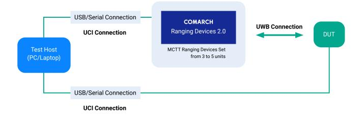
MCTT operates on a traditional PC/laptop with a USB connection to a set of Comarch MCTT Ranging Devices 2.0. According to the latest FiRa MAC Test Specification 2.0, the required number of MCTT Ranging 2.0 is between 3 and 5 units. Communication between MCTT Ranging Devices 2.0 and the Device Under Test (DUT) is carried over UWB.
