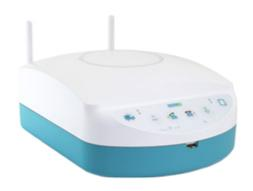
Comarch HMA (Home Medical Assistant) collects data from peripheral devices by wireless connection, and transmits it to the Remote Medical Care Center. Because it can be used with a wide range of medical sensors, including those provided by outside firms, Comarch HMA is a universal device which can constitute a home measuring station and, thanks to videoconferencing, voice- or text-communication, can be the fastest way to estabilish contact between patient and physician.
