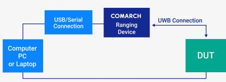
This is a plug and play solution. MCTT works on a traditional PC with a USB connection to a Comarch ranging device. Communication is done over UWB. For the purpose of development and preparation of ATL (Authorized Test Lab) for certification, we also deliver sample devices. Ask our sales rep for more details.
